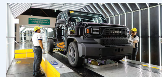
Toyota Motor Philippines line team conducts final inspection of the all-new Next Generation Tamaraw in Santa Rosa Plant
